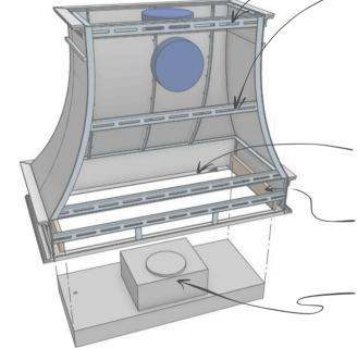
• MOUNTING STRAPS | horizontal straps across the back of the hood in at least 2 locations (may have more). These straps are perforated along the entire length to enable them to cover the full range of potential mounting location studs. Hood is mounted by lagging thru these straps into the framing in your wall.
